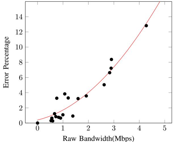
Figure 4. Error percentage and raw-bandwidth(Mbps) for a pair of eight senders and eight receivers communicating a payload of “11111111...1”.
