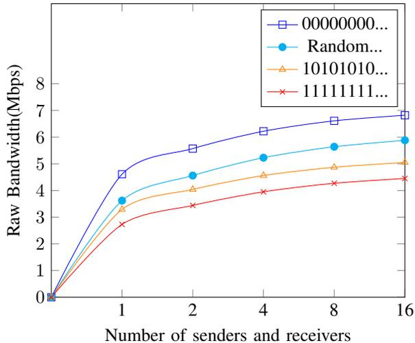
Figure 3. Raw bandwidth for different data payloads with various sender-receiver configurations.
