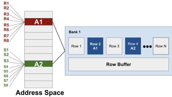
Figure 1. Eight sender (S1 to S8) and receiver (R1 to R8) processes communicating over one DRAM bank. All the senders share and access address A1 and all the receivers share and access address A2. Both A1 and A2 are mapped to two different DRAM rows but one DRAM bank.
