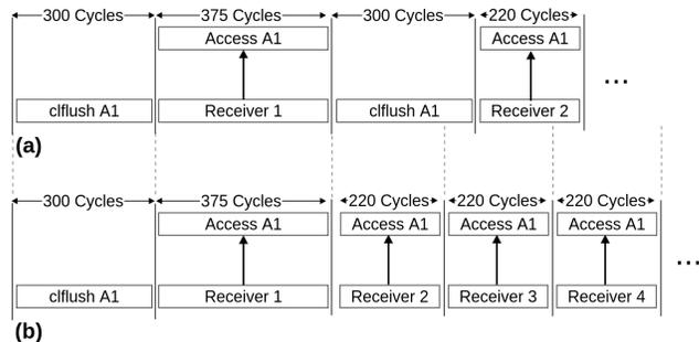
Figure 2. Timing diagram for a payload of “0000...”. (a) Covert Channel on a conventional cache and (b) proposed covert channel on a TimeCache.
